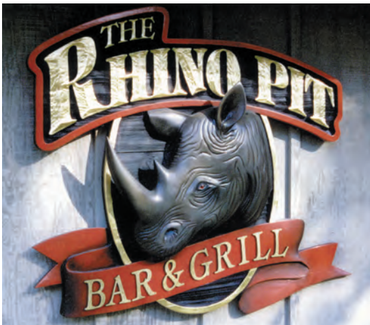
Here, a sign company provided both fabrication and design services. This 40 by 50-in. wall sign incorporates a sandblasted and carved redwood panel with carved Sign Foam® artwork and 23K gold lettering with a blended enamel finish.
